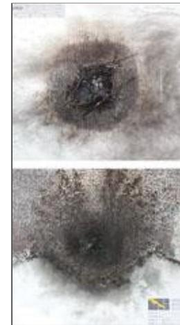
Source: APCMTwo lightning strike test panels: the one at top shows burn-through that resulted from lack of lightning strike protection; the panel at bottom, protected by Strike Guard LSP prepreg, shows only localized surface damage.
